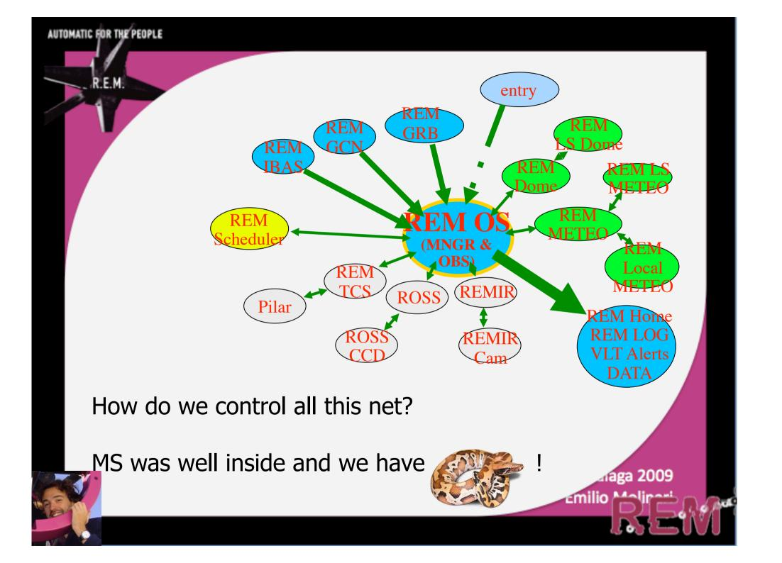
A full basket of pythons running every 2/5 minutes to feed telemetry of telescope and instruments, check status, send alarms.
